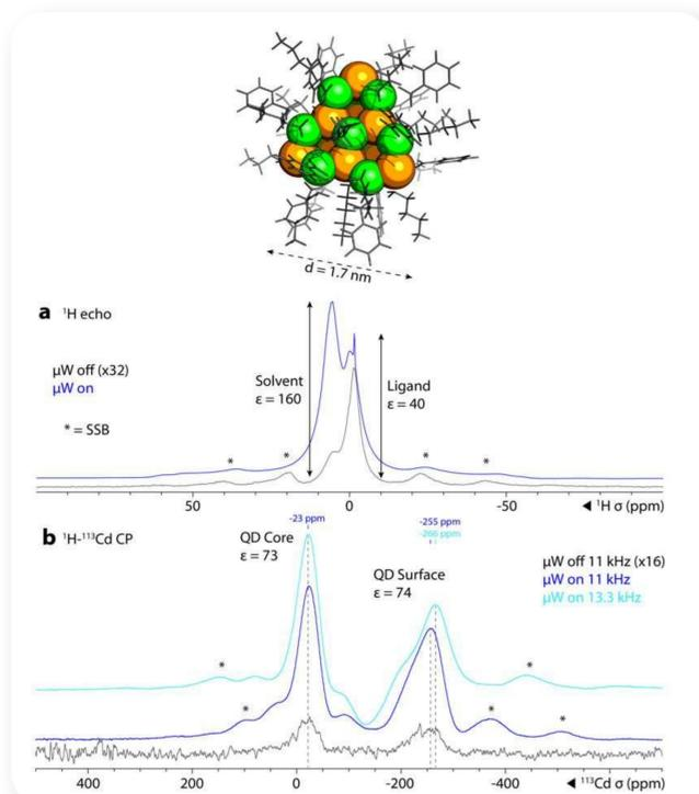
Fig. 1 (a)  $^1\text{H}$  and (b)  $^{113}\text{Cd}$  DNP spectra of 1.7 nm QD colloidal samples show distinct chemical shifts and anisotropies for core and surface cadmium sites. Surface site shifts are sensitive to MAS frequency. In collaboration with J. Owen, Columbia University.
