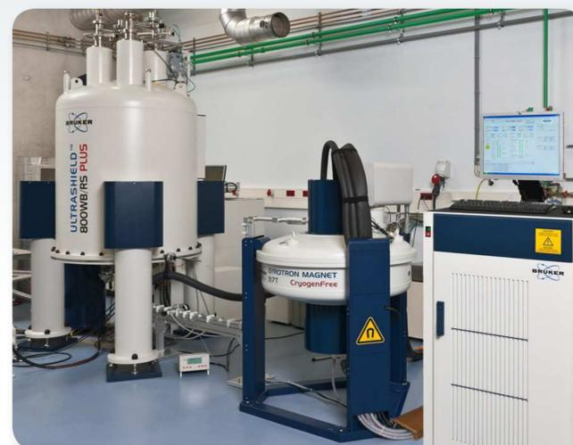
Fig. 2 527 GHz DNP Spectrometer at the University of Utrecht, The Netherlands. Left to right: 800 WB NMR magnet, microwave transmission line, second-harmonic cryogen-free gyrotron tube and magnet, control system.
