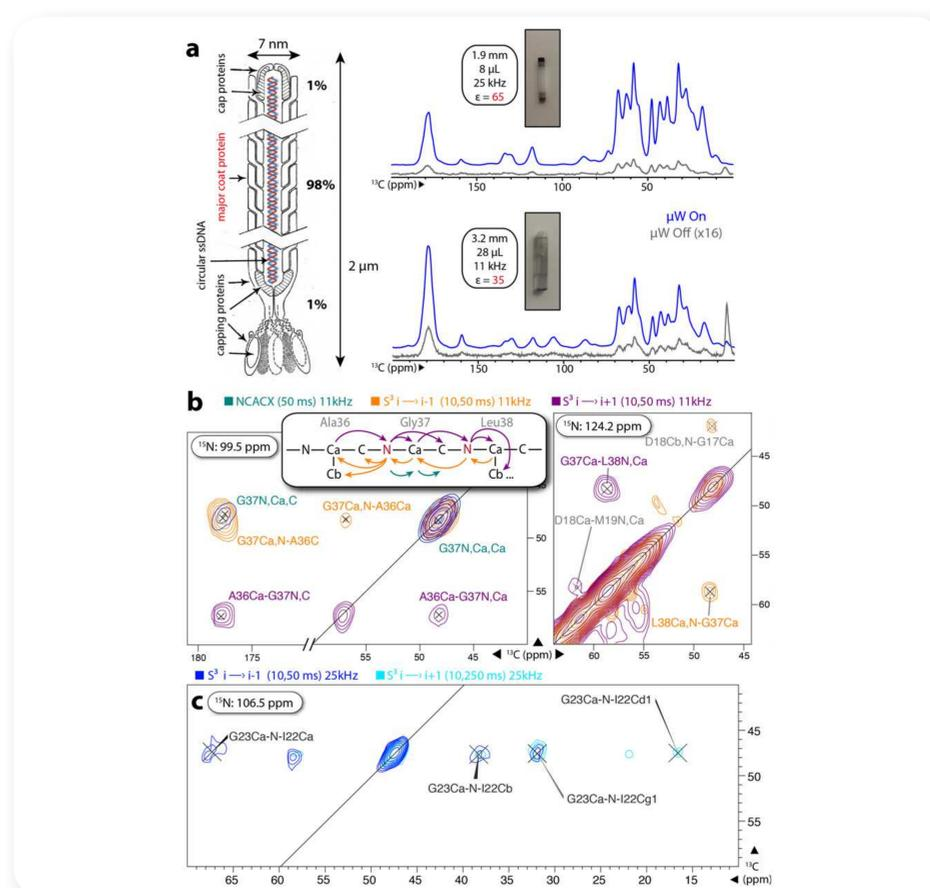
Fig. 3 (a) Intact Pf1 bacteriophage samples yield promising DNP enhancements in both 3.2 mm and 1.9 mm rotors. (b) Assignments of the Pf1 major coat protein are simplified using the sequential sidechain-sidechain correlation ( $S^3$ ) technique. (c) 25 kHz MAS improves the resolution of DNP spectra, enables long-range inter-residue polarization transfers, and is helpful for extending assignments. I. Sergeev et al. 2016 PNAS submitted.
